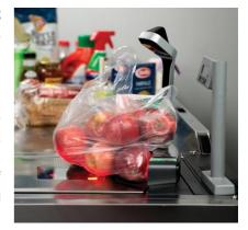
Both scanners are equipped with Datalogic's patented "Green Spot" technology. When a bar code is read, a green spot is projected on the code informing the user of a good read, an advantageous feature for busy supermarkets operating multiple checkout lanes in close proximity to one another.
